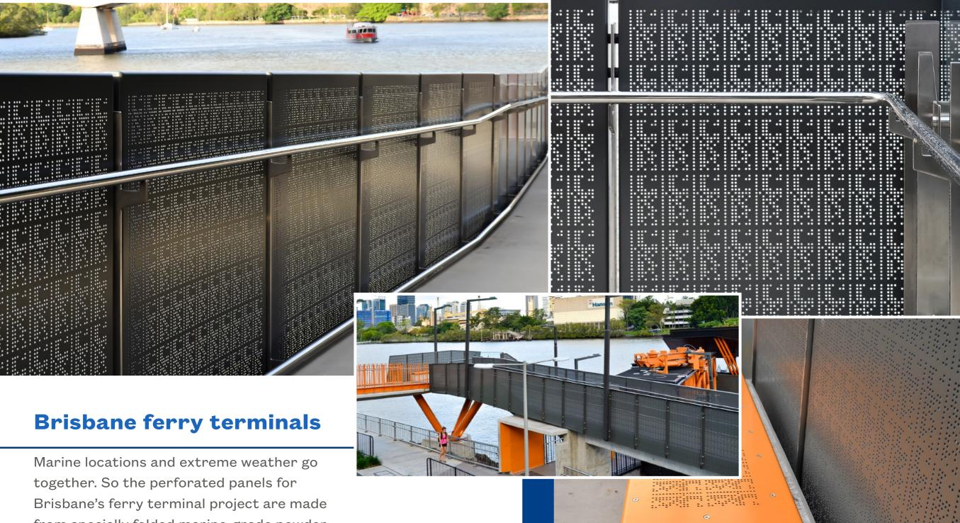
from specially folded marine-grade powdercoated aluminium, resulting in smooth sailing for passenger accessibility and safety.
